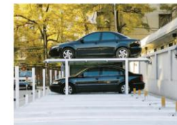
Four vertical columns type The stable frame structure encounters even force. Chain drive.
